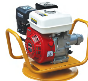
KF-ZB50 VIBRATOR: KF-ZB50 发动机: 汽油 168-1 燃烧方式: 风冷, 单缸, 四冲程 发动机功率, 最大 KW (HP): 4.7 (6.5) Engine: Gasoline 168-1 Combustion Way: Air-cooled, Single Cylinder, Four Stroke Engine Power: Max KW (HP): 4.7 (6.5) Weight (kg): 22
